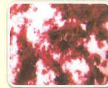
Activated sludge from conventional process Dispersed & poor setting
