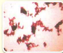
Activated sludge from BASS™ process Denser & separate flocs
